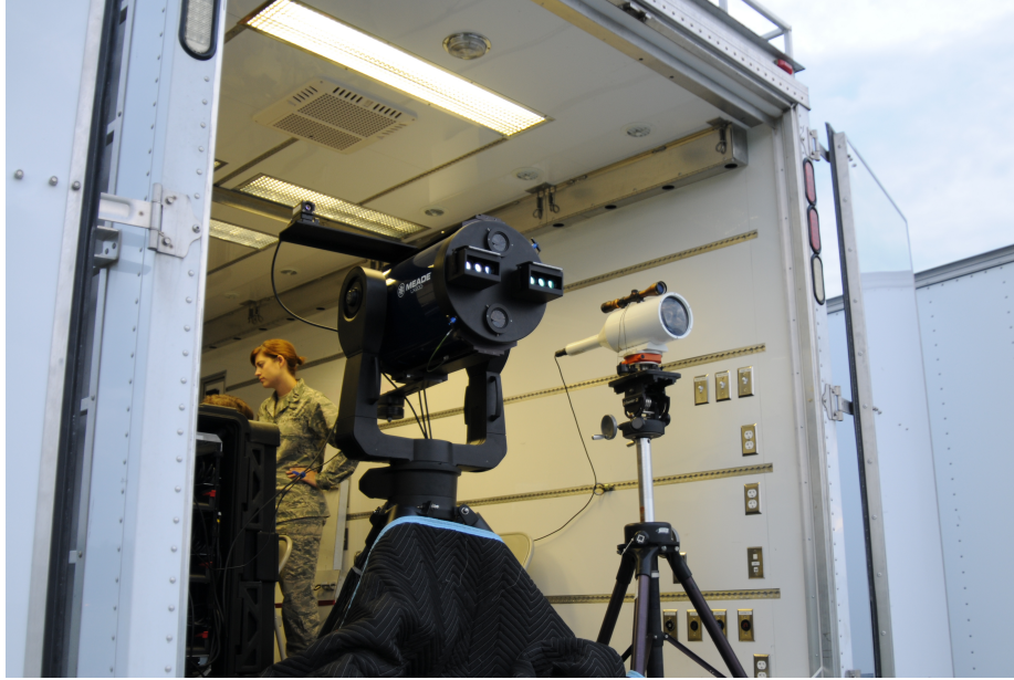
Figure 24. The trailer from which the lasers operated when located out doors. The apertures for each laser are at the front of the black cylindrical object pointing out of the trailer.
