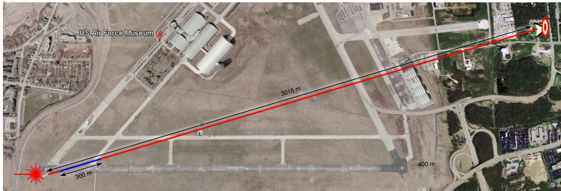
Figure 27. Experiment geometry for the 15 July 2009 test. For this test, the observer was located almost directly below the beam. The 300 m field of view is representative of the 31.75 cm reflecting telescope, which was used for most of the observations on 15 July.
