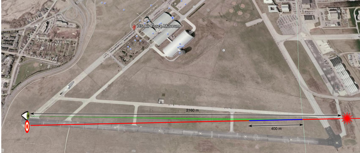
Figure 28. Experiment geometry for the 17 July 2009 test. The source is denoted by a laser symbol, the target by a bulls-eye, and the observer by an eyeball. The observer's field of view is identified by a blue line along the laser beam path. The 400 m field of view is representative of the 10.1 cm refracting telescope, which was used for most of the observations on 17 July.
